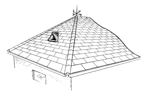
Figure 4 Example of an owl entrance hole through a hipped roof
